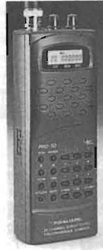
Realistic PRO-50 20 canali 68-88, 137-174 380-512 MHz AM-FM
