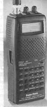
Realistic PRO-60 200 canali 30-512, 760-999 Hyperscan AM-FM-FMW
